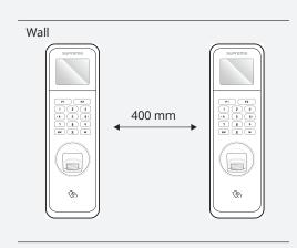
• When using a mobile access card, install devices maintaining a minimum distance of 1 m between devices to avoid RF interference.
